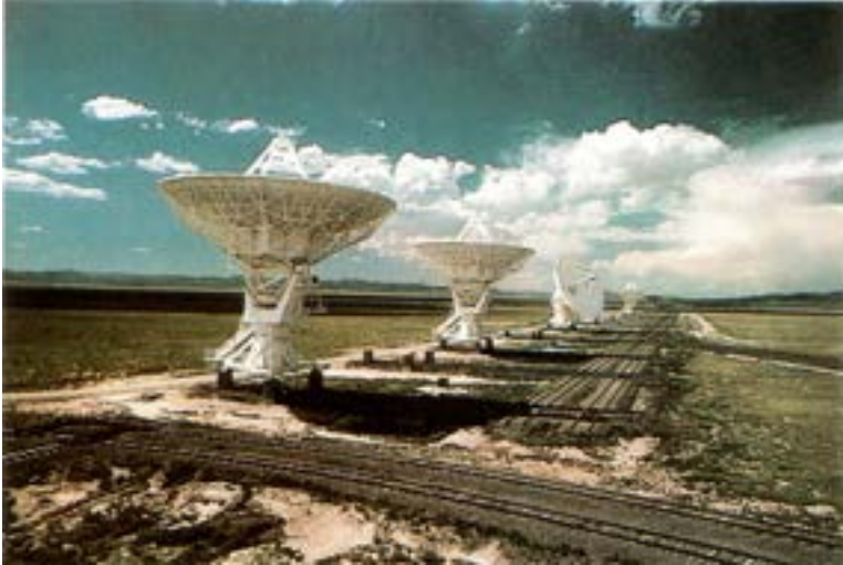
A few of the radio telescopes of the Very Large Array, Socorro, New Mexico, operated by the National Radio Astronomy Observatory. The telescopes move on railway tracks; their separation determines the resolution of the resulting radio image.
