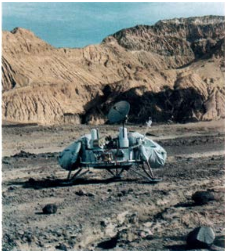
The Viking Lander, in simulation in Death Valley, California. Between the two turrets containing the television cameras is the magazine holding the still-unfurled sample arm.
