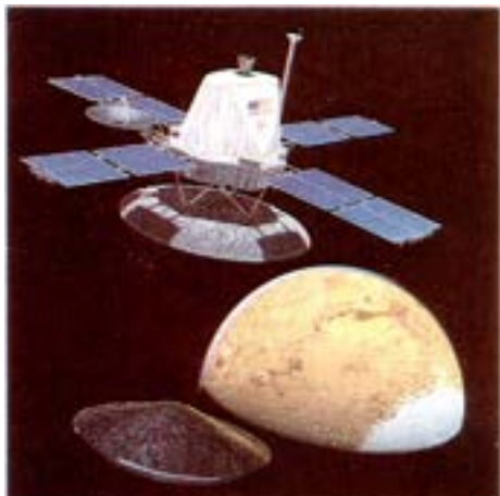
A Viking Lander, wrapped in its aeroshell ablation shield ( bottom ), detaches from the Orbiter and enters the thin Martian atmosphere. Both are in orbit about Mars, thousands of kilometers below, its polar cap prominent. Painting by Don Davis.
