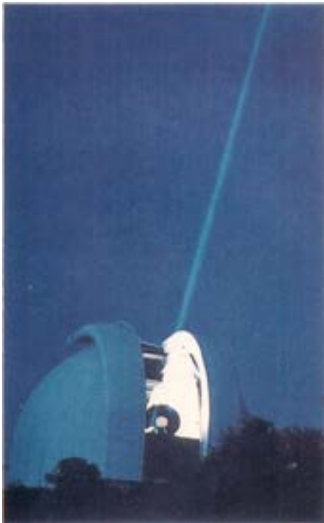
Laser beam directed at retroreflectors emplaced on the lunar surface. The telescope is the 82-inch reflector of McDonald Observatory, University of Texas.
