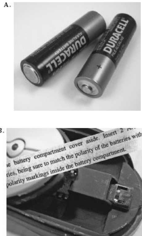
FIGURE 4.2. Cylindrical Battery: Where Constraints Are Needed. Figure A shows the traditional cylindrical battery that requires correct orientation in the slot to work properly (and to avoid damaging the equipment). But look at Figure B, which shows where two batteries are to be installed. The instructions from the manual are shown as an overlay to the photograph. They seem simple, but can you see into the dark recess to figure out which end of each battery goes where? Nope. The lettering is black against black: slightly raised shapes in the dark plastic.
