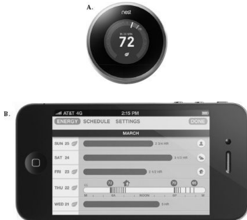
FIGURE 2.6. A Thermostat with an Explicit Conceptual Model. This thermostat, manufactured by Nest Labs, helps people form a good conceptual model of its operation. Photo A shows the thermostat. The background, blue, indicates that it is now cooling the home. The current temperature is 75°F (24°C) and the target temperature is 72°F (22°C), which it expects to reach in 20 minutes. Photo B shows its use of a smart phone to deliver a summary of its settings and the home’s energy use. Both A and B combine to help the home dweller develop conceptual models of the thermostat and the home’s energy consumption. (Photographs courtesy of Nest Labs, Inc.)
