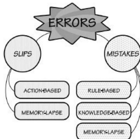
FIGURE 5.1. Classification of Errors. Errors have two major forms. Slips occur when the goal is correct, but the required actions are not done properly: the execution is flawed. Mistakes occur when the goal or plan is wrong. Slips and mistakes can be further divided based upon their underlying causes. Memory lapses can lead to either slips or mistakes, depending upon whether the memory failure was at the highest
