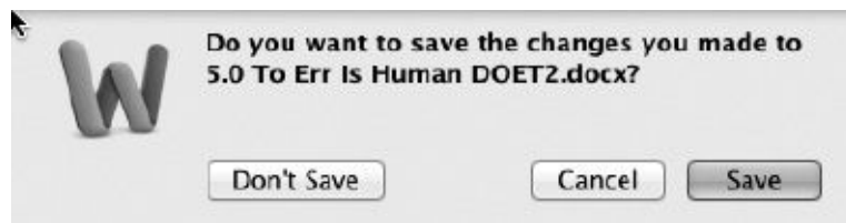
FIGURE 4.6 A Lock-In Forcing Function. This lock-in makes it difficult to exit a program without either saving the work or consciously saying not to. Notice that it is politely configured so that the desired
