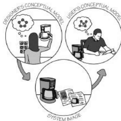
FIGURE 1.11. The Designer's Model, the User's Model, and the System Image. The designer's conceptual model is the designer's conception of the look, feel, and operation of a product. The system image is what can be derived from the physical structure that has been built (including documentation). The user's mental model is developed through interaction with the product and the system image. Designers expect the user's model to be identical to their own, but because they cannot communicate directly with the user, the burden of communication is with the system image.
