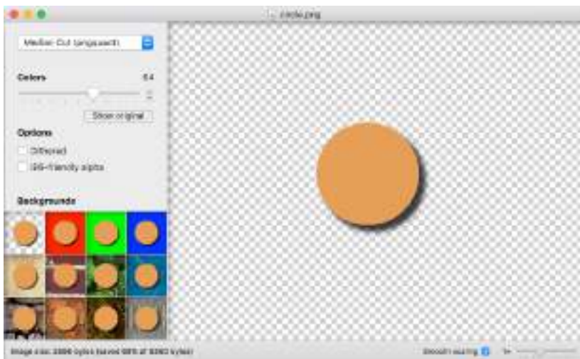
FIGURE 24-17. The ImageAlpha compression tool (Mac only) turns PNG-24s with alpha transparency into PNG-8s while retaining multiple transparency levels.
