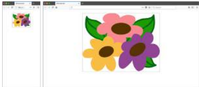
FIGURE 25-17. The SVG scales automatically and proportionally with the size of its container.
