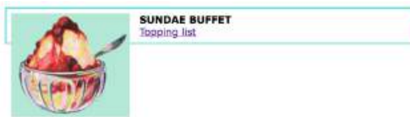
FIGURE 15-9. The containing element does not expand to accommodate the floated image as indicated by its blue border.
