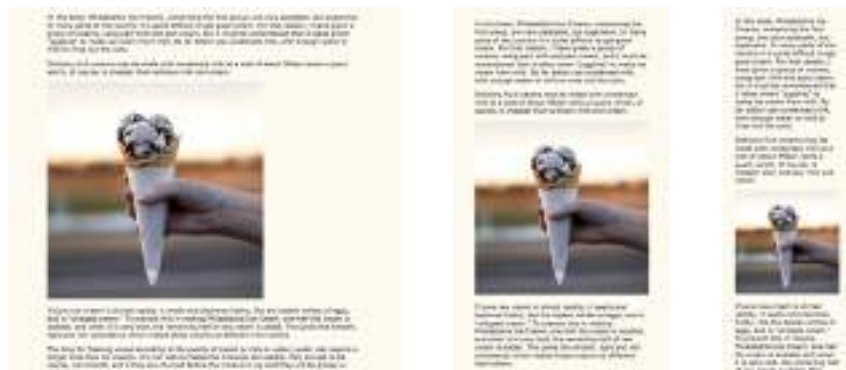
FIGURE 17-4. Setting the max-width of inline images allows them to shrink to fit available space but not grow larger than actual size.
