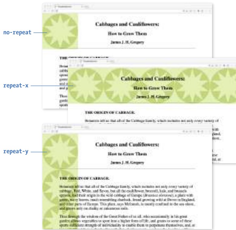
FIGURE 13-20. Turning off automatic tiling with no-repeat (top), applying horizontal-axis tiling with repeat-x (middle), and applying vertical-axis tiling with repeat-y (bottom).
