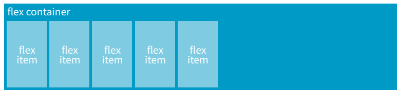
FIGURE 16-2. Applying the flex display mode turns the child elements into flex items that line up along one axis. You don’t need to do anything to the child elements themselves.
