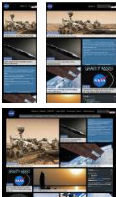
FIGURE 3-3. A responsive site's layout changes based on the size of the browser window.
