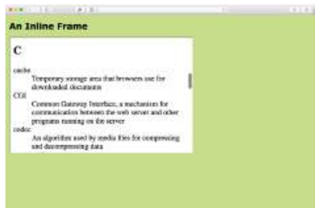
FIGURE 10-1. Inline frames (added with the iframe element) are like a browser window within the browser that displays external HTML documents and resources.
