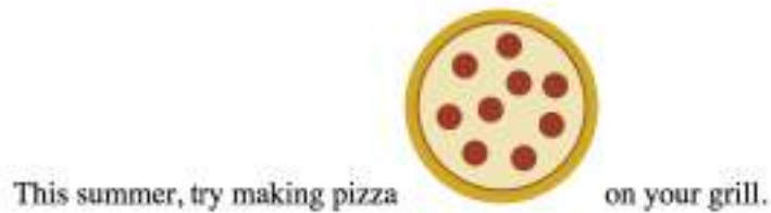
FIGURE 7-8. This pizza image is an SVG made up of 11 circle elements. Instead of an img element, the SVG source code is placed right in the HTML document with an svg element.
