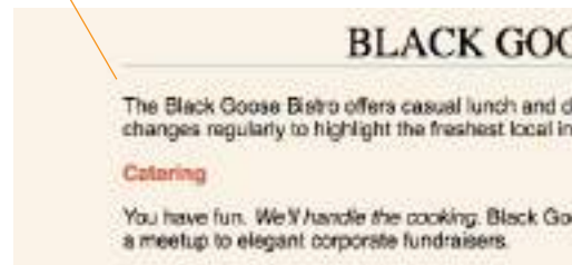
FIGURE 4-18. A missing end bracket makes the browser think the following characters are part of the tag, and therefore the headline text doesn't display.
