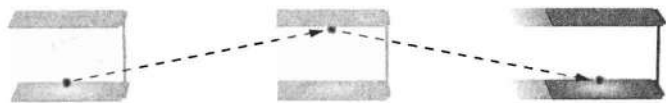
Figure 2.3 From our perspective, the photon in the sliding clock travels on a diagonal path.
